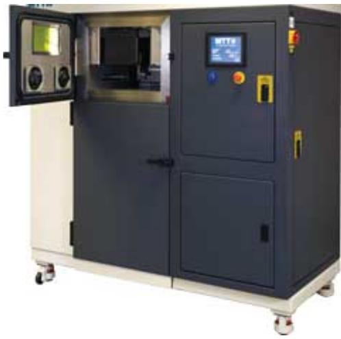
**The third-generation SLM 250 System from MMT Group (now part of Renishaw). Enhancements over previous models include variable powder delivery, ultra-low oxygen content in the build atmosphere, and a safe-change filter system to minimize user materials-contact. Image courtesy MTT/Renishaw.**
