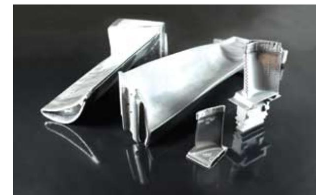
**This Direct Metal Deposition rebuilt turbine blade squealer-tip was done on a POM Group system. Sizes vary from 50mm to 600mm (H). *Image courtesy POM Group.***
