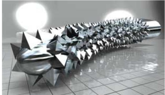
**A bone rasp under development by Within Technologies for manufacture on an EOS laser-sintering system. The part represents a particular challenge for AM building, because the surface is covered with 2x2mm pyramids whose orientation keeps changing to match the overall shape of a helix.**
